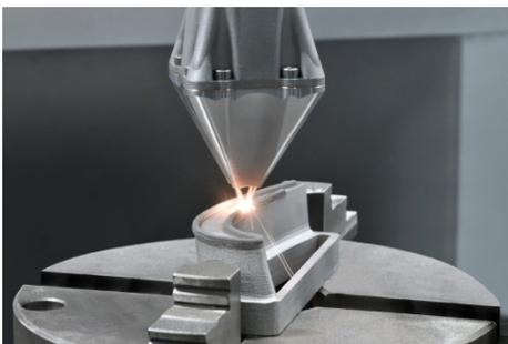
Example for repairing of damaged blade.
